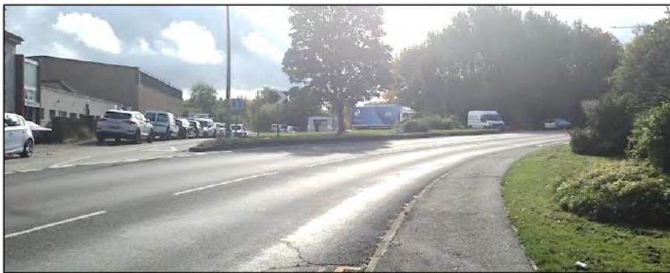
3.3.11 It is proposed that this service road be converted to a 3.5m southbound bus lane (as requested by Officers) with removal of on street parking and a widened footway. The existing direct accesses currently served by the service road will be retained. This is illustrated opposite using a further extract from drawing 47444-5501-004.
